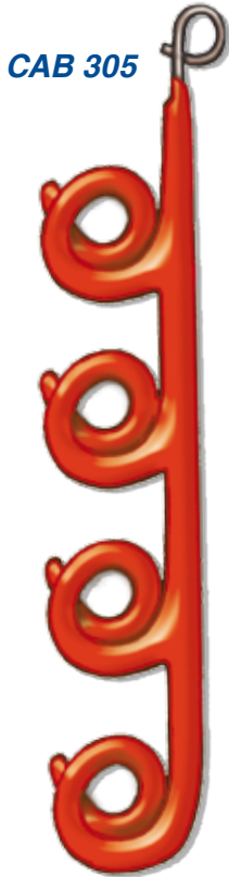
CAB 305 has four 1" (25mm) diameter closed spiral loops. 1/2" (13mm) diameter top loop has closed spiral design which prevents dislodging of hanger from beltline chain or other support after installation. .156 wire (4mm), 11-3/4" (298mm) long.
